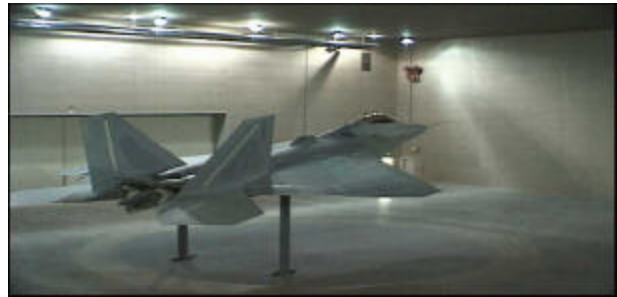
Figure 11: Indoor Signature Test Facility
