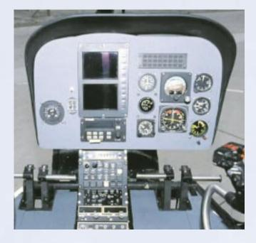
The VEMD (Vehicle and Engine Multifunction Display) is a fully duplex equipment allowing the display on LCD screen of 3 operating modes which are:
