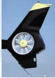
Third generation of Fenestron with airfoil and 8 asymmetrical blades spacing for low noise emission.
