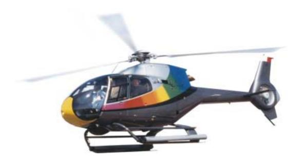
The EC 120 B is the first light single engine helicopter to incorporate the latest technologies available such as VEMD (Vehicle and Engine Multifunction Display), Spheriflex type rotor head, a new generation fenestron and the latest TURBOMECA ARRIUS engine.
