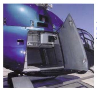
The luggage compartment is able to contain up to 5 large suitcases. When the helicopter is configured for internal freight transport, the cabin area plus luggage compartment make loading and unloading effortless thanks to an unobstructed cabin and a flat floor.
