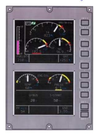
The VEMD (Vehicle and Engine Multifunction Display) is a fully duplex equipment which displays on LCD screen 3 operating modes :
