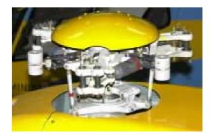
The main rotor generates the lift and the traction transferred to the helicopter. During flight, it allows the helicopter to be controlled in roll and pitch in conjunction with the tail rotor (yaw).
